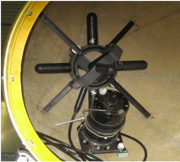
Figure 3. Homing transducer array mounted in the nose cone. Below it is the 675 kHz bottom avoidance sonar.
